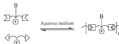
Scheme 1. Schematic representation of the formation of polycationic dynamic covalent polymers from functionally complementary monomers; B represents a nucleobase.
